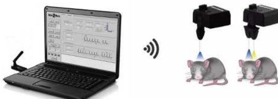
Fig. 1. Schematic Diagram of Wireless Programmable Optogenetic Experiment Instrument
